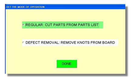
Switch between regular mode and defect removal mode with this screen.
