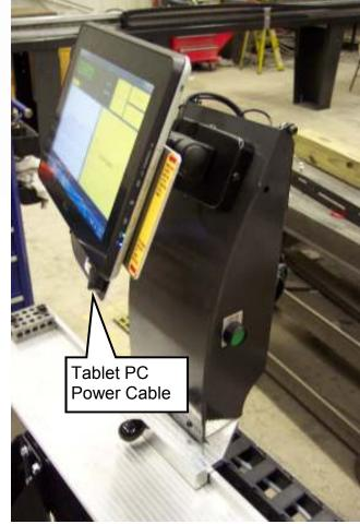
Step 3) Locate the main power cable that runs through the flexible track on the back of the machine and plug it into a s110 VAC outlet. Make sure the power strip on the back of the tablet enclosure is turned on. Then turn on the enclosure power and then power up the PC tablet using the controls labeled below.
