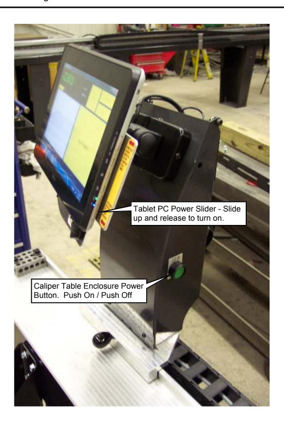
Once the tablet PC is booted up, double click the Caliper Table icon on the Windows desktop. The software will load and you should see the screen below. Use the knob on the front of the slide to move the carriage against the stop block and press the ZERO the Scale button on the screen. Your caliper table is now ready to use. The callouts below indicate other functions available on the main screen. The following pages explain the Log File and Setup buttons.
