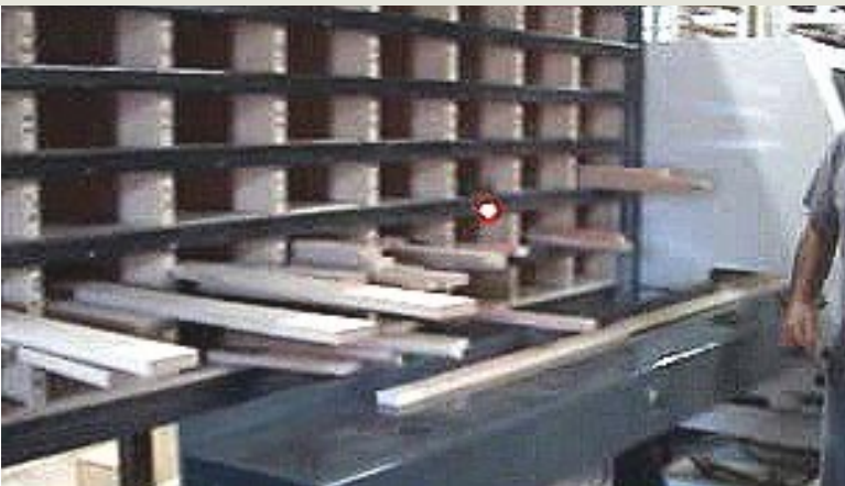
RazArray - LEDs indicate in which bin parts belong.
