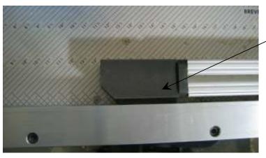
Top View of RazorGage Miter Stop shown with fingers hidden in groove in machine fence.
