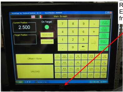
The NEC 17" Touch Screen RGX00409 has NEC printed on the upper left corner and the buttons are mounted in a module located on the bottom center of the bezel.
