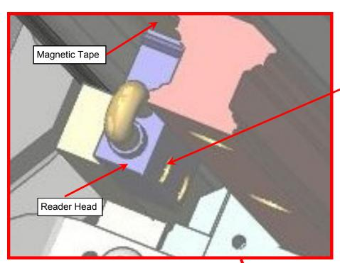
Use 2.5mm L-shaped allen wrench with short arm of the 'L" ground down to access the two screws that mount the linear encoder reader head. Slip a strip of notebook paper between the reader head and the mag tape, hold the reader head against the paper, tighten the screws, and remove the paper.
