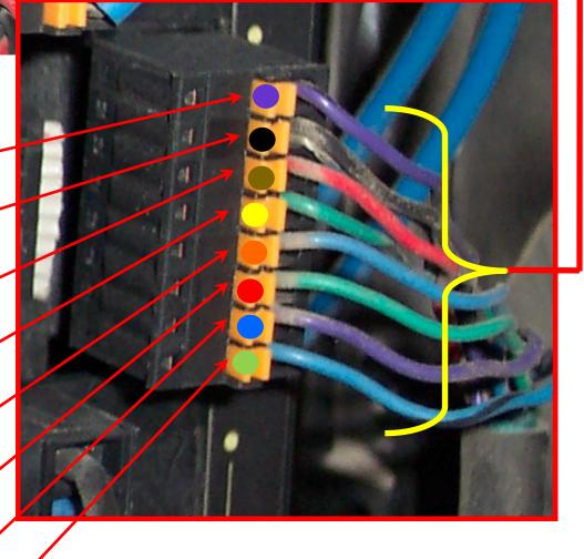
Check to make sure the correct color wire is in the correct terminal. Press the orange button to release a wire. Remove and re-insert each wire ensuring that the terminal is clamping on copper and not clamping on the insulation.
