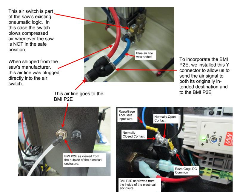
The BMI P2E has one Normally Open and one Normally Closed contact. In this case the air signal is absent when the saw is up (safe). Since the RazorGage is looking for a closed contact when the saw is safe, we tied the RazorGage Tool Safe input wire to the Normally Closed contact.
