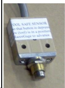
Down Cut Saw - Switch detects that saw is up.
