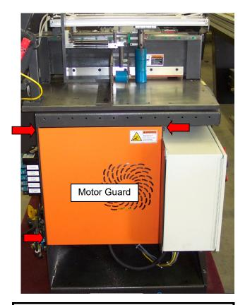
To adjust how high the saw blade extends, first lock out power and air to the machine and then remove the motor guard by removing the screws indicated at left by the red arrows.
