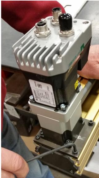
4) Loosen drive assembly mtg. screws.
