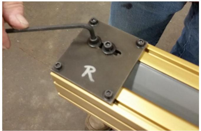
20) Tighten idler slide screws.
