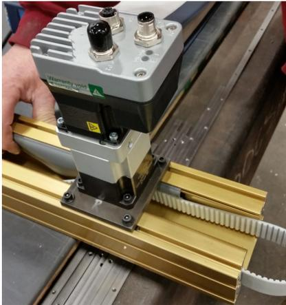
12) Slide the drive assembly inboard about 6".
