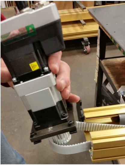
10) With idler removed, drive assembly will slide out.
