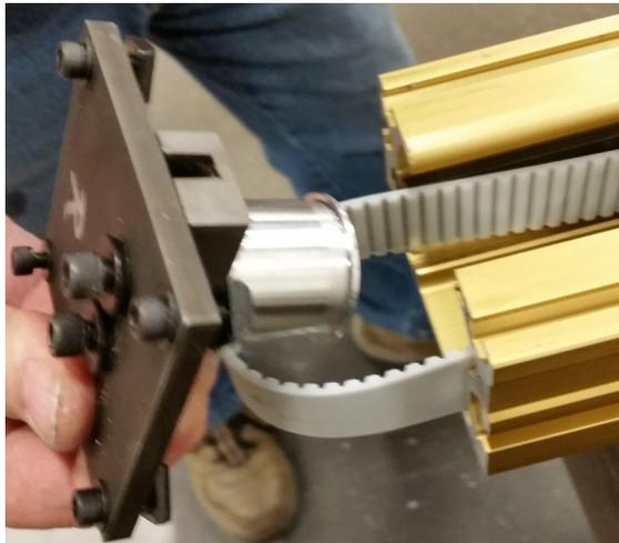
8) Using belt slack gained by sliding drive assembly inboard, slide idler out & remove.
