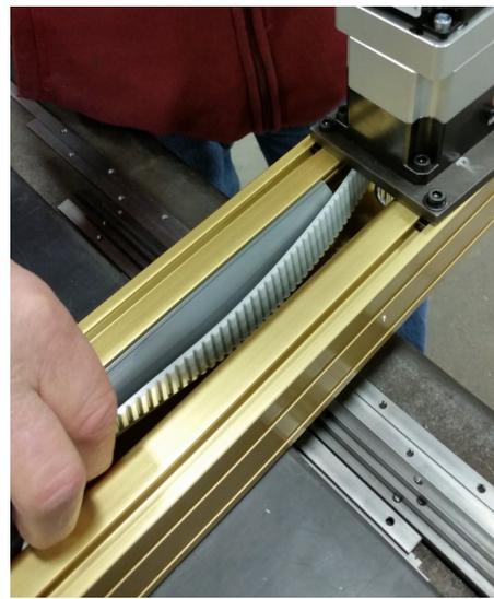
11) As before, tuck about 12" of seal under the belt on the new motor end.
