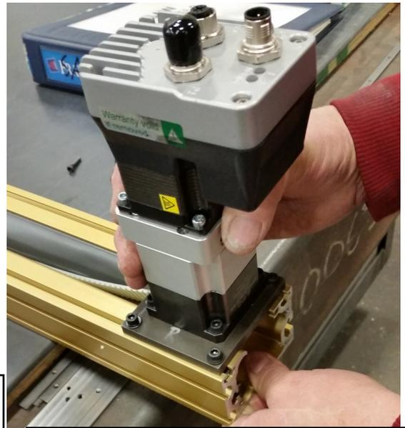
14) Position drive assembly flush with end and tighten mounting screws TIGHT!
