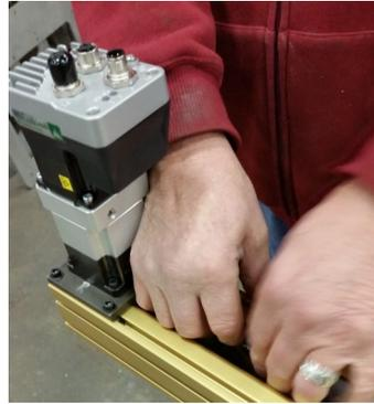
3) Tuck about 12" of seal under belt on motor end.
