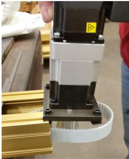
11) On the end drive assy. is moving to, pull belt loop out and slide the drive assembly into the T-Slots.
