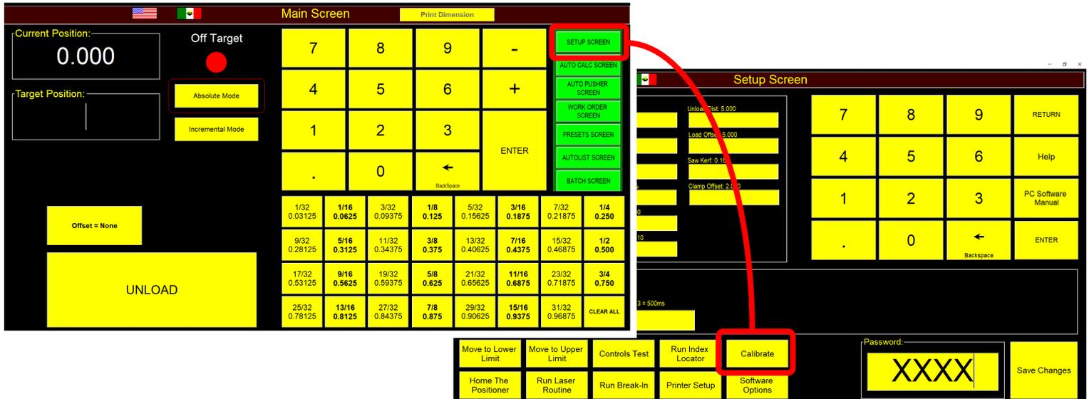
**Saw Kerf:** When using the RazorGage as a pusher the Home Offset will only affect the accuracy of the first trim cut. Part length accuracy is a factor of the scale factor and the kerf. If all parts are equally inaccurate simply adjust the kerf. If short parts are accurate and long parts are not or vice versa then adjust the scale factor in step two of the Calibration Wizard accessed from the Calibrate Home Offset button. Step 2 password is 5239
