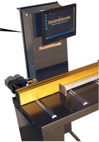
The Mini Enclosure MUST be flush with this edge when mounted to the RazorGage extrusion. Otherwise the carriage could hit the enclosure during homing.
