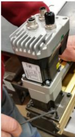
4) Loosen drive assembly mtg. screws.
