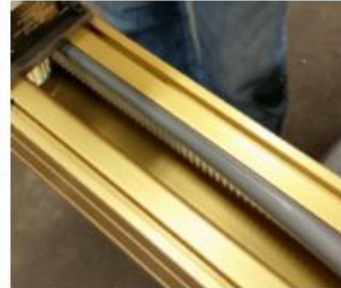
3) Tuck about 12" of seal under belt on motor end.
