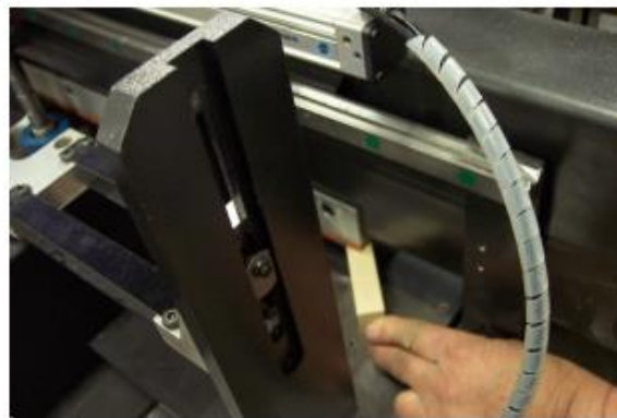
Step 3 for All Cyclone 600 Saws: Manually raise the top clamp and place a spacer under it to hold it up off the table.
