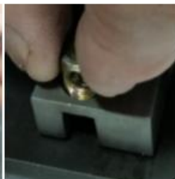
9) Move brass threaded plug and tensioning screw to opposite side of idler block.
