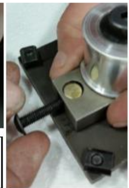
9) Move brass threaded plug and tensioning screw to opposite side of idler block.
