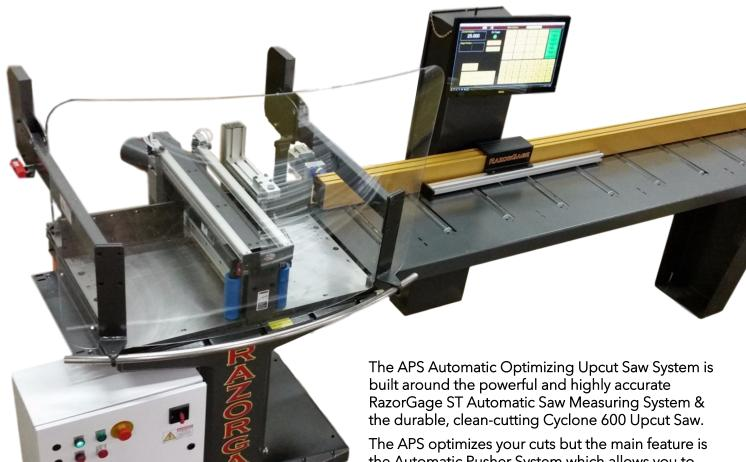
the Automatic Pusher System which allows you to push "Go" and stand back. The automatic saw does the work and allows one person to both feed the saw
