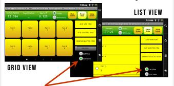
**Preset Grid Scaling Slide Bar** allows you to easily adjust the Preset button size or you can change to list view to scroll through your Presets using the swipe feature.
