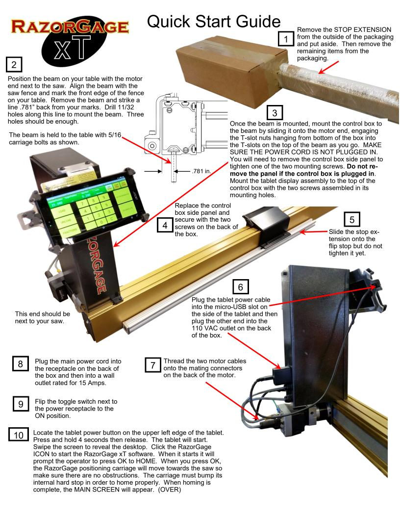
With the positioner at the home position, slide the stop extension to a point about an inch from the saw blade cutting plane and tighten the locking screw.
