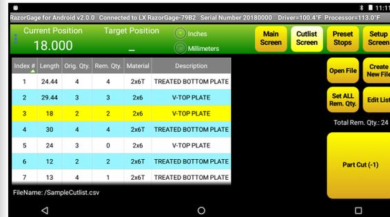
**Create your cutlists** at the machine or email a cutlist over a WiFi network. The Android has tremendous storage capacity, so you are not limited to saving only small cut lists. Cutlists can also be restored to original quantities after use or even multiplied if you want to make several "kits" of parts at once.
