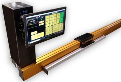
The RazorGage ST Automatic Saw Measuring System is at the heart of our product line. Whether you use the ST as an automatic pusher or a measuring stop, this digital measuring fence can be used with a chop saw, upcut saw, downcut saw, drill press, haunching, notching and punching machines.
