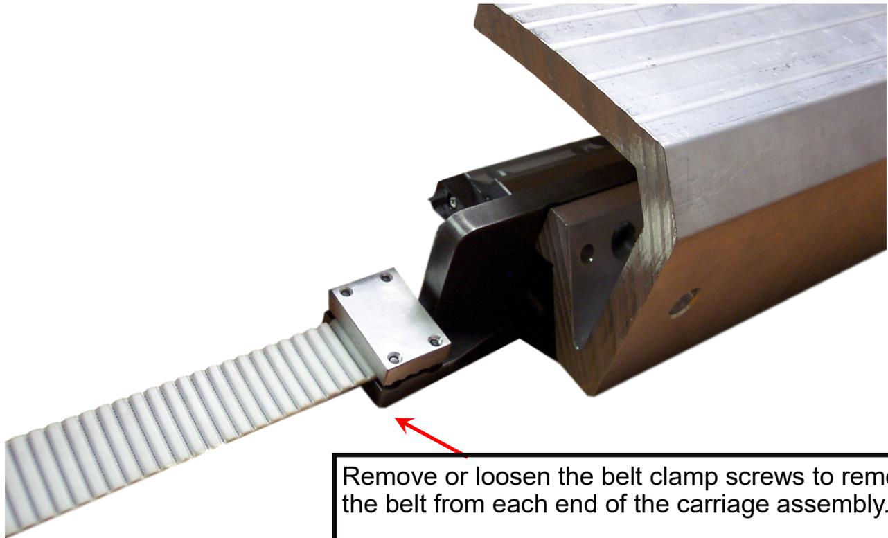
Remove or loosen the belt clamp screws to remove the belt from each end of the carriage assembly.
