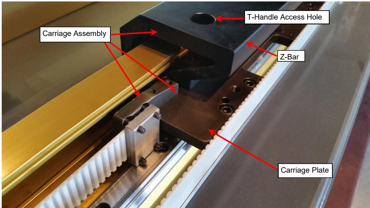
If you need to remove the Z-Bar, use a T-Handle allen wrench to access the socket head cap screws that secure the Z-Bar to the carriage plate. The Z-Bar is pinned to the carriage plate so one must remove it by gently working it off the pins once the screws are removed.
