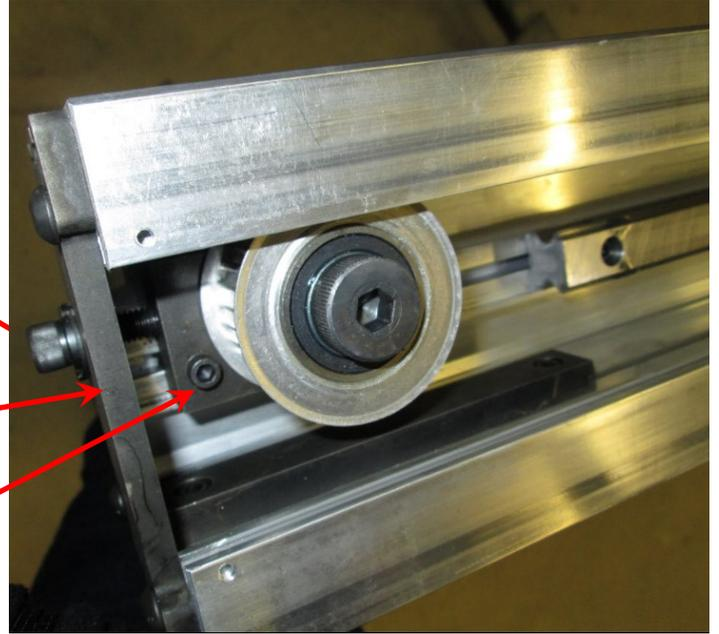
2) Loosen the two screws that hold the idler block and slide the idler block toward the motor to relieve tension on the belt.
