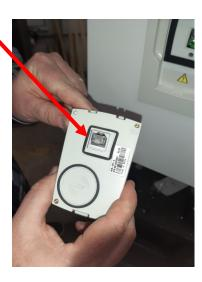
Step 2: Open the saw cabinet door and make sure the data cable on the display door mount is secure and also secure at the frequency drive. The data cable will look like an ethernet cable. If the problem persists there could be a problem with the door mount or the data cable.
