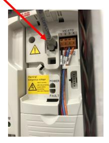
The display can also be plugged directly into the drive. This will allow you to operate the saw until you replace the data cable
