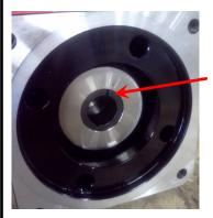
After removing the MDrive, look inside the gearhead to make sure the sleeve is in place and that the slot in the sleeve is not lined up with the set screw you loosened in step one. If it is, rotate it inside the bore so that the slot is not aligned with the set screw.
