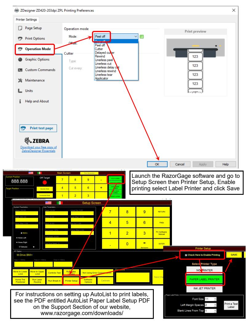
After you have enabled printing go back into printer setup and perform a test print to ensure that everything is configured properly
