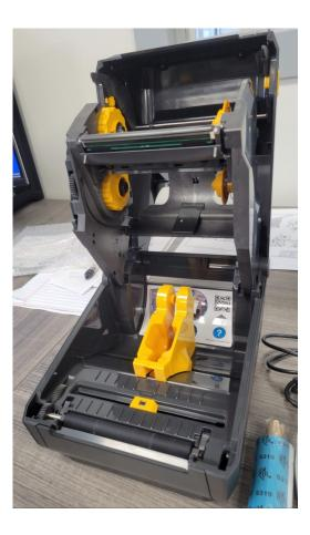
Load label paper as shown. Ensure it is underneath the yellow tabs.
