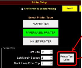
This should print a test label similar to the one shown here. If the label is off center then adjust the Left Margin Spaces setting by changing the value clicking save, going back into printer setup and printing another test label.
