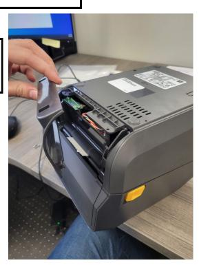
Push dispenser down until flush with bottom of printer.
