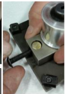
9) Move brass threaded plug and tensioning screw to opposite side of idler block.
