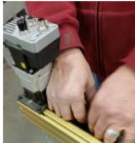
3) Tuck about 12" of seal under belt on motor end.
