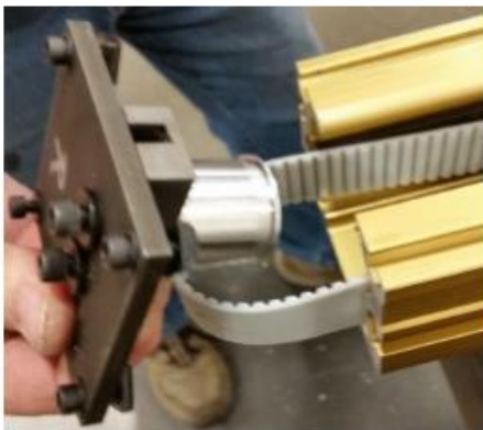
8) Using belt slack gained by sliding drive assembly inboard, slide idler out & remove.
