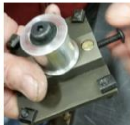
9) Move brass threaded plug and tensioning screw to opposite side of idler block.
