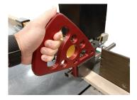
The Face Frame Scribe package can be included on new RazorGage RG3 with AutoList Optimizing Software and it can easily be added to existing RazorGage PC based ATs and RazorGage ST / AutoList systems. The package includes the software and the scribing tool.
