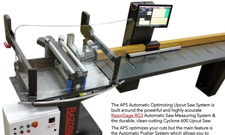
The APS optimizes your cuts but the main feature is the Automatic Pusher System which allows you to push "Go" and stand back. The automatic saw does the work and allows one person to both feed the saw and stack the finished parts, with no interruption.
