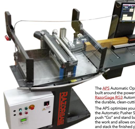
The APS Automatic Optimizing Upcut Saw System is built around the powerful and highly accurate RazorGage RG3 Automatic Saw Measuring System & the durable, clean-cutting Cyclone 600 Upcut Saw.
