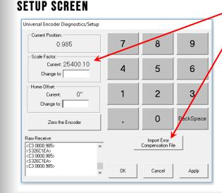
The scale factor is the number of encoder counts per inch. Adjust the Scale Factor to improve accuracy.
